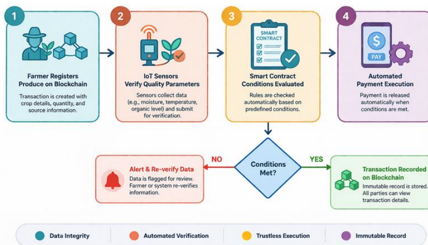
Figure 2: Smart Contract Workflow in Agricultural Transactions Depicting Automated Verification, Conditional Evaluation, and Immutable Recording of Transactions
